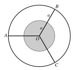
A uniform disc, of mass 4m and radius a, and a uniform ring, of mass m and radius 2a, each have centre O. A wheel is made by fixing three uniform rods, OA, OB and OC, each of mass m and length 2a, to the disc and the ring, as shown in the diagram. Show that the moment of inertia of the wheel about an axis through A, perpendicular to the plane of the wheel, is  $42ma^2$ . [5]
