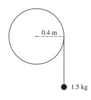
A uniform disc of radius 0.4 m is free to rotate without friction in a vertical plane about a horizontal axis through its centre. The moment of inertia of the disc about the axis is  $0.2 \text{ kg m}^2$ . One end of a light inextensible string is attached to a point on the rim of the disc and the string is wound round the rim. The other end of the string is attached to a particle of mass 1.5 kg which hangs freely (see diagram). The system is released from rest. Find
