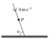
A small smooth ball P is moving on a smooth horizontal plane with speed  $4 \,\mathrm{m\,s^{-1}}$ . It strikes a smooth vertical barrier at an angle  $\alpha$  (see diagram). The coefficient of restitution between P and the barrier is 0.4. Given that the speed of P is halved as a result of the collision, find the value of  $\alpha$ . [5]
