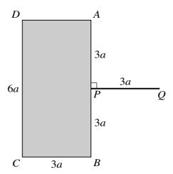
An object is formed by attaching a thin uniform rod PQ to a uniform rectangular lamina ABCD. The lamina has mass m, and AB = DC = 6a, BC = AD = 3a. The rod has mass M and length 3a. The end P of the rod is attached to the mid-point of AB. The rod is perpendicular to AB and in the plane of the lamina (see diagram). Show that the moment of inertia of the object about a smooth horizontal axis  $l_1$ , through Q and perpendicular to the plane of the lamina, is  $3(8m + M)a^2$ . [4]
