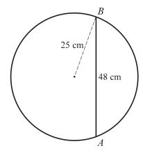
A frame consists of a uniform circular ring of radius  $25 \,\mathrm{cm}$  and mass  $1.5 \,\mathrm{kg}$ , and a uniform rod of length  $48 \,\mathrm{cm}$  and mass  $0.6 \,\mathrm{kg}$ . The ends A and B of the rod are attached to points on the circumference of the ring, as shown in the diagram. Find the distance of the centre of mass of the frame from the centre of the ring.
