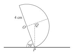
A uniform solid hemisphere, with centre O and radius 4 cm, is held so that a point P of its rim is in contact with a horizontal surface. The plane face of the hemisphere makes an angle of  $70^{\circ}$  with the horizontal. Q is the point on the axis of symmetry of the hemisphere which is vertically above P. The diagram shows the vertical cross-section of the hemisphere which contains O, P and Q.
