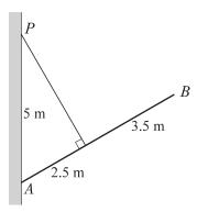
A uniform beam AB has length 6 m and mass 45 kg. One end of a light inextensible rope is attached to the beam at the point 2.5 m from A. The other end of the rope is attached to a fixed point P on a vertical wall. The beam is in equilibrium with A in contact with the wall at a point 5 m below P. The rope is taut and at right angles to AB (see diagram). Find
