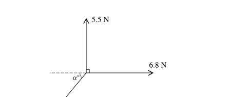
Three coplanar forces act at a point. The magnitudes of the forces are 5.5 N, 6.8 N and 7.3 N, and the directions in which the forces act are as shown in the diagram. Given that the resultant of the three forces is in the same direction as the force of magnitude 6.8 N, find the value of  $\alpha$  and the magnitude of the resultant. [4]
