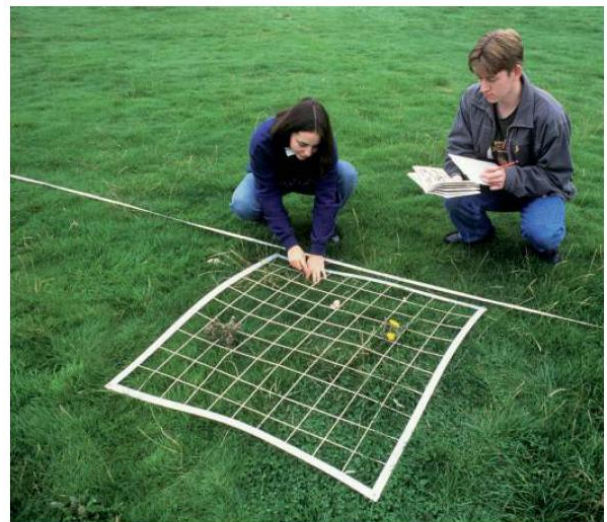
Figure 18.9 Estimating percentage cover. This 1 m 2 quadrat is divided into 100 small squares to make it easier to make the estimation for each species.
