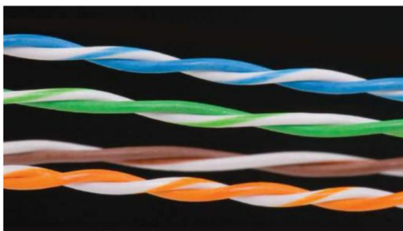
Figure 20.14 Twisted wire-pairs in a computer network.
