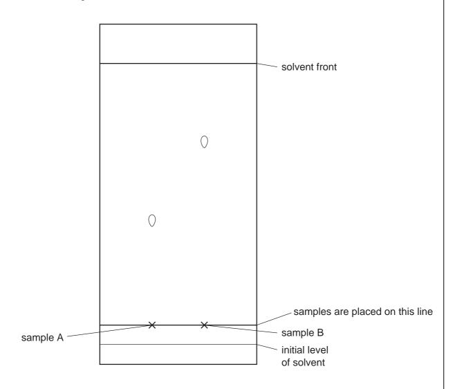
(i) The  $R_f$  value of a sample = <u>distance travelled by sample</u> distance travelled by solvent front
