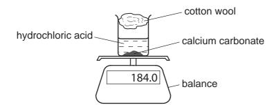
The beaker was placed on a balance and the mass of the beaker and contents recorded every minute.
