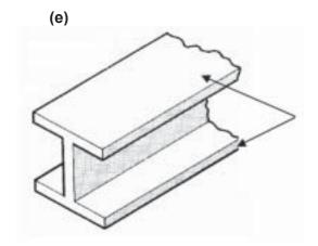
The web of the **I** beam resists shear (1), the flanges resist bending (1) Clear drawing (1)
