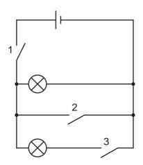
Which switches must he close to light both lamps?
