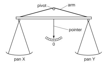
Four masses (in total) are placed on the pans, with one or more on pan X and the rest on pan Y.
