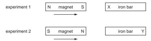
Which magnetic poles are induced at X and at Y?
