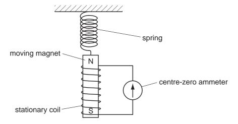
What does the ammeter show when the magnet repeatedly moves slowly up and down?
