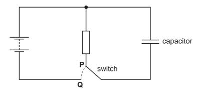
What happens to the capacitor when the switch is at **P** and when it is at **Q**?
