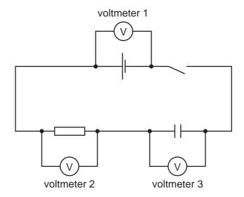
Immediately after the switch is opened, which voltmeters will read zero?
