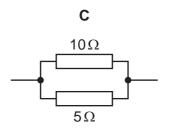
The total resistance is less than  $5\Omega$ .
