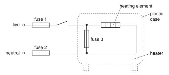
Which of the fuses are correctly placed?
