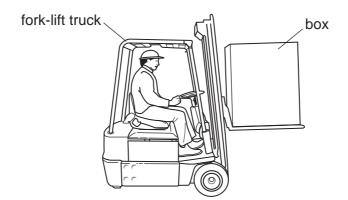
The force exerted by the fork-lift truck on the box is 3500 N upwards.
