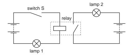
When switch S is closed, the relay operates. What is the state of the lamps?
