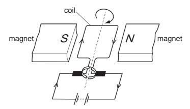
Which change will make the motor rotate more quickly?
