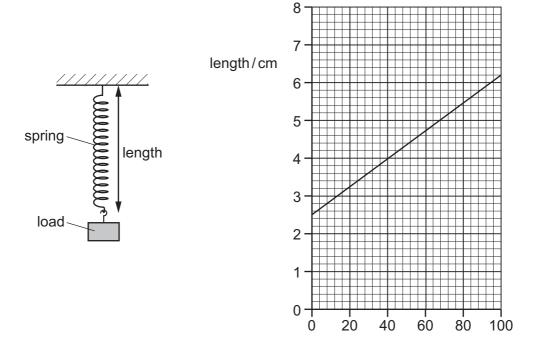
What is the extension of the spring when a load of 40 N is applied to it?
