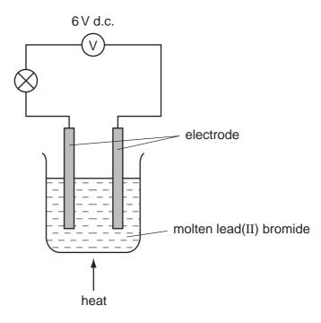
The bulb goes out soon after the heat is removed.
