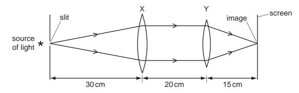
What are the correct values for the focal lengths of X and of Y?
