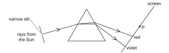
A thermometer placed at P shows a large temperature rise.
