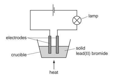
The crucible needs to be heated for the bulb to give out light.
