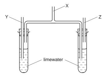
Where does air enter and leave the apparatus?
