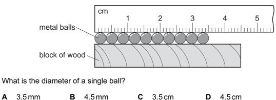
**29** A ruler and a block of wood are used to find the diameter of some identical metal balls.
