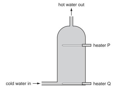
When only heater Q is switched on, it takes a very long time to heat the tank of water to the required temperature of 60 °C.
