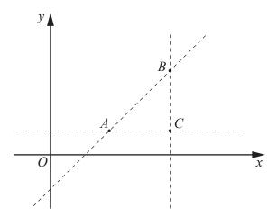
A is the point (5, 2) and B is the point (9, 6). AC is parallel to the x-axis. CB is parallel to the y-axis. The equation of the line AB is x - y = 3.
