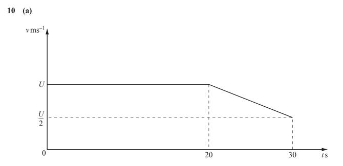
The diagram shows part of the velocity-time graph for a particle, moving at  $v \,\mathrm{ms}^{-1}$  in a straight line, *t* s after passing through a fixed point. The particle travels at  $U \,\mathrm{ms}^{-1}$  for 20 s and then decelerates uniformly for 10 s to a velocity of  $\frac{U}{2} \,\mathrm{ms}^{-1}$ . In this 30 s interval, the particle travels 165 m.
