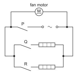
The fan motor has a power rating of 0.10 kW and the heaters each have a rating of 0.40 kW. The cost of electricity is 8.0 cents / kW h.
