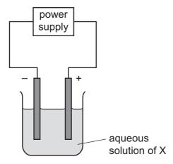
Hydrogen is produced at the cathode and chlorine is produced at the anode.
