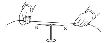
An electric current is switched on in the wire and the compass needle is deflected.
