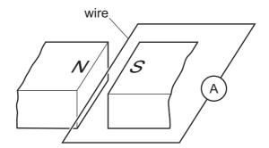
The wire is moved downwards, towards the bottom of the page. A current is induced in the wire.
