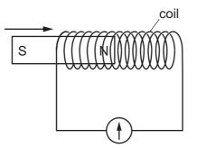
The needle of the galvanometer moves.
