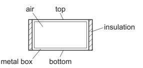
A scientist investigates the thermal conductivity of air. She measures how quickly thermal energy passes between the top and bottom of the box.
