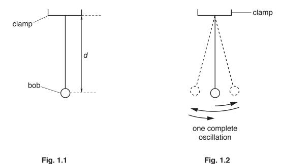
(a) The student adjusts the length of the pendulum until the distance *d*, measured to the centre of the bob, is 50.0 cm. State one precaution that you would take to obtain the length of 50.0 cm as accurately as possible.
