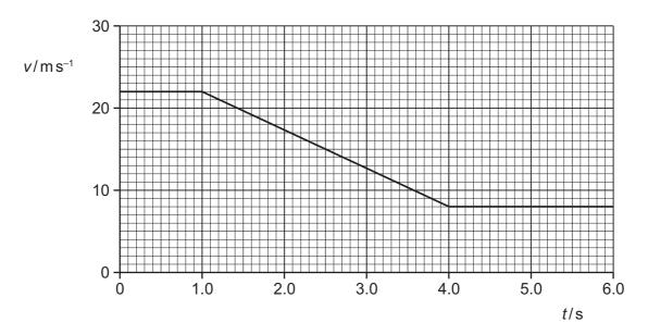
The brakes of the car are applied from  $t = 1.0 \,\mathrm{s}$  to  $t = 4.0 \,\mathrm{s}$ .
