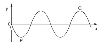
What is the phase difference between points P and Q on the wave?
