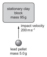
The mass of the pellet is 5.0 g and the mass of the clay block is 95 g.
