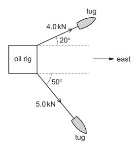
The tensions in the towing cables are 4.0 kN and 5.0 kN.
