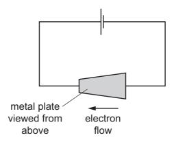
Electrons move clockwise around the circuit.
