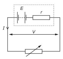
The variable resistor is adjusted so that *I* increases.
