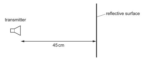
The emitted waves have a frequency of 1.00 GHz. A stationary wave is produced with a node at the transmitter and a node at the surface.
