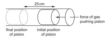
How much work is done by the gas on the piston when it moves through a distance of 25 cm?
