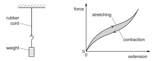
The force–extension curve for contraction is below the force–extension curve for stretching.
