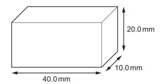
The calipers can measure with an absolute uncertainty of  $\pm 0.1$  mm.
