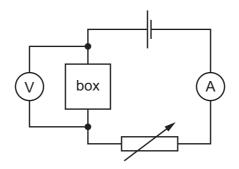
The variable resistor is adjusted and measurements are taken to determine the I-V characteristic for the box, as shown.
