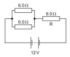
What is the power dissipated in resistor R?
