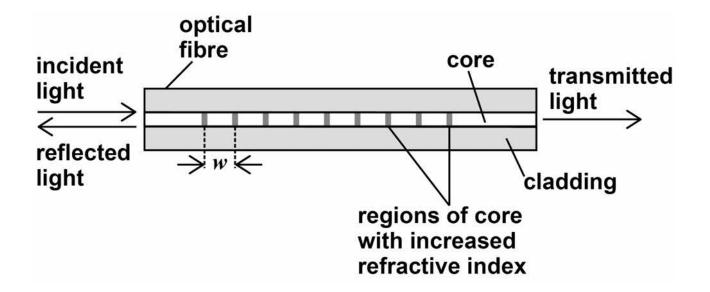
A maximum intensity of the reflected light is produced due to superposition of the light reflected from each of the regions with increased refractive index in the core. This maximum intensity occurs at a particular wavelength  $\lambda_R$ .
