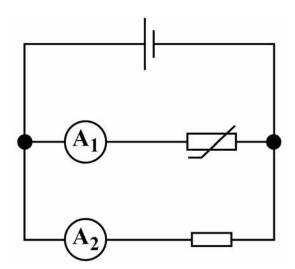
The cell has a constant electromotive force and negligible internal resistance. Readings from the two ammeters are taken.
