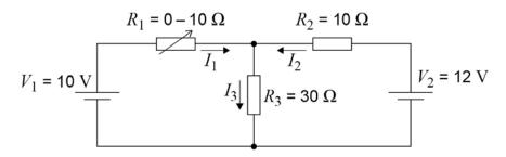
$R_1$  is a variable resistor with a resistance that varies between 0 and 10  $\Omega$ .
