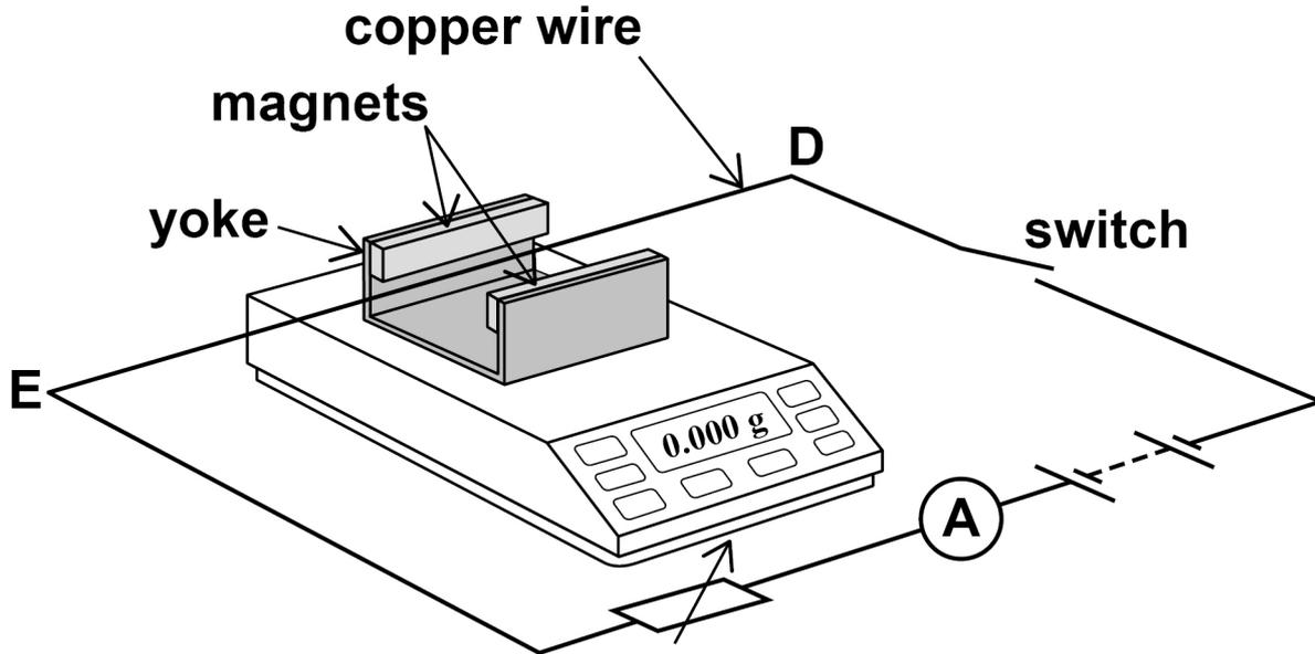
The magnets produce a uniform horizontal magnetic field in the region between them. A copper wire DE is connected in the circuit shown in FIGURE 2 and is clamped horizontally at right angles to the magnetic field.
