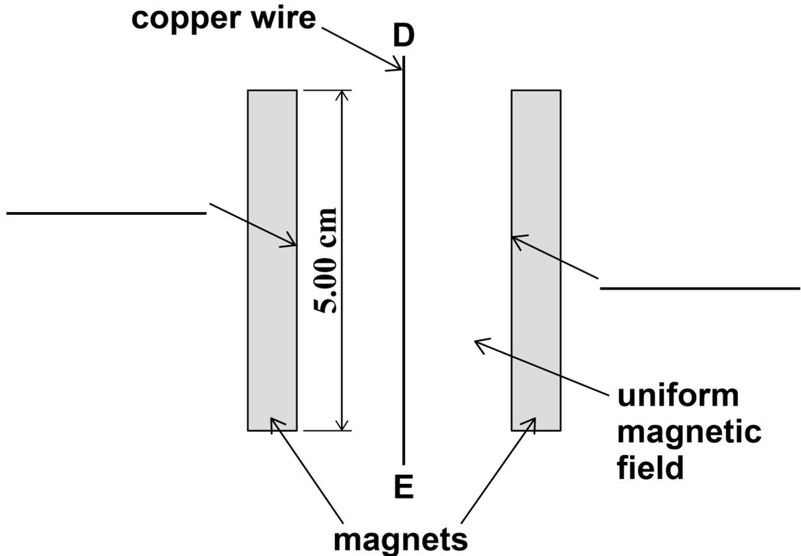
When the apparatus is assembled with the switch open, the reading on the electronic balance is set to 0.000 g. This reading changes to a positive value when the switch is closed.
