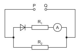
Under which circumstances does the ammeter show a reading other than zero?
