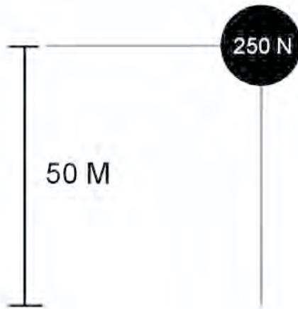
The 250N boulder shown in the diagram above possesses PE, which can be stated in equation form below.
