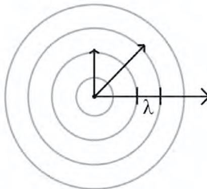
As we look at the event from above, the curvature of each wave front changes with distance. As the wave front moves further from the center it becomes less and less curved. The arrows are called *rays* and represent the straight line direction in which a single point on the wave front is moving. Rays are always perpendicular to the wave front.
