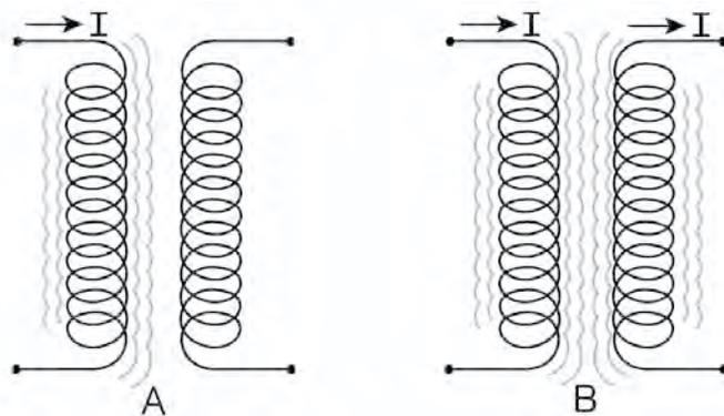
Transformers that reduce the applied voltage are called step-down transformers. Those that increase the applied voltage are called step-up transformers. The ratio of the input voltage and the output voltage is determined by the ratio of the number of turns of wire in the primary and the secondary sides of the transformer.
