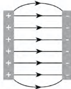
The only place the field lines are *not* parallel is at the edges of the parallel plate.
