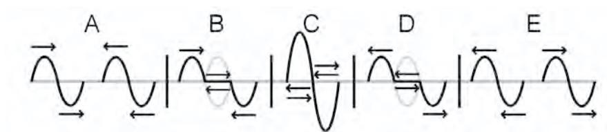
Diagrams A through E show two identical waves,  $x$  and  $y$ , traveling in opposite directions on a string.
