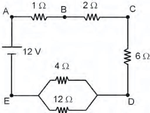
The electrical circuit shown has 1 ampere of current flowing in it. Answer the questions about the parts of the circuit listed between the points below by choosing the letter that correctly represents the quantity in question.
