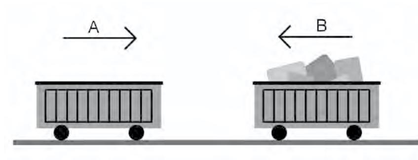
A freight train is being assembled in the freight yard. An empty car (A) with a mass of 4000 kg is moving along the track with a velocity of 1.5 m/s. Another car (B) is completely loaded, has a mass of 16,000 kg, and is moving in the opposite direction at 10 m/s. The boxcars collide, couple together, and move off. What is the velocity and direction of movement of the two boxcars?
