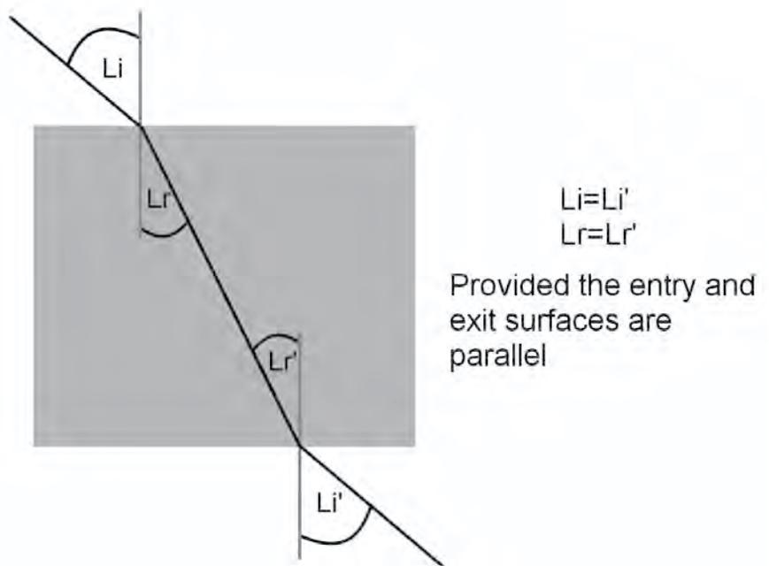
At the air/plastic boundary, the light ray bends (refracts) toward the normal when the light ray passes into the plastic. The ray moves in a straight line while in the plastic until it reenters the air. At the plastic/air boundary the light ray bends (refracts) away from the normal.
