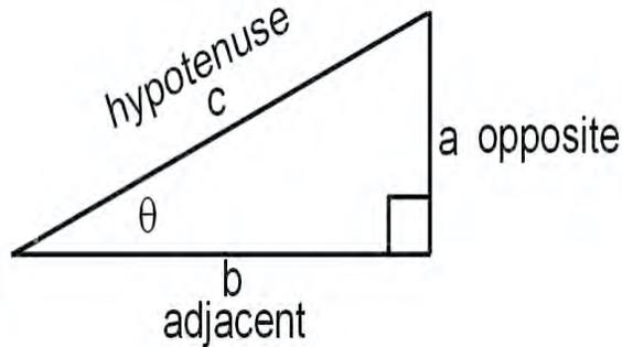
The right triangle above is labeled according to convention. The side opposite the  $90^\circ$  angle is called the hypotenuse and is labeled  $c$ . The side beside the smaller of the remaining two angles is called the adjacent side  $b$ , and the side across from the smaller angle is called the opposite side  $a$ .
