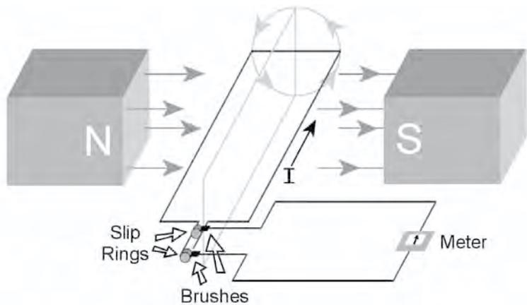
The current and voltage produced in the AC generators is not steady as in DC systems. Both current and voltage increase and decrease each time the loop of wire in the magnetic field turns a full 360°. The diagram below shows a comparison between AC and DC voltages.
