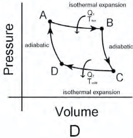
During processes AB and BC, positive work is done, but during processes CD and DA, negative work is done. The net work done by the system is the area enclosed by ABCDA.
