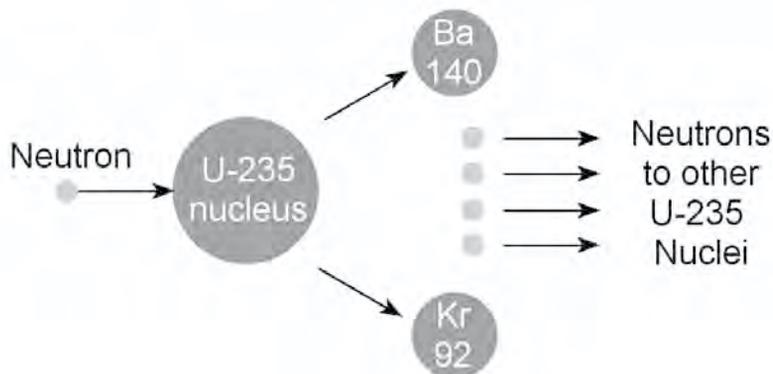
The diagram above illustrates the process through which the uranium nucleus is split to produce the two daughter nuclei and four neutrons. We can calculate the energy released in the reaction by finding the change in mass between the reactant nucleus and neutron and the products.
