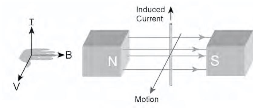
The direction of an electric current induced into a wire can be predicted by using the right-hand rule.
