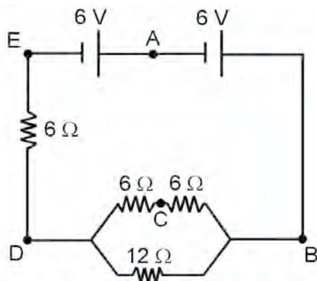
13. Through which point does half the total current pass?
