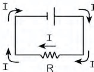
When more than one resistor is in a series circuit, the value of each resistor is added together to give the total resistance.
