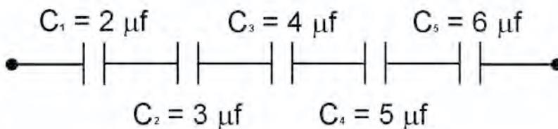
$$\frac{1}{C_t} = \frac{1}{C_1} + \frac{1}{C_2} + \frac{1}{C_3} + \frac{1}{C_4} + \frac{1}{C_5}$$
