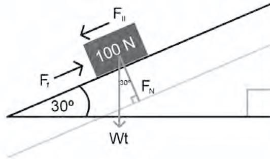
The diagram above shows a block sliding down a raised plane at a constant rate. The force parallel ( $F_{||}$ ) is the applied force, the weight ( $wt$ ) of the object acts directly toward the earth, the normal force ( $F_N$ ) acts directly out of the surface, and the frictional force ( $F_f$ ) opposes the motion of the block.
