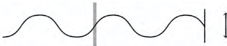
The rope vibrates on the vertical axis, and the meter stick is oriented on the vertical axis. If we change the orientation of the stick to the horizontal axis, the vertical vibrations in the rope strike the horizontal meter stick.
