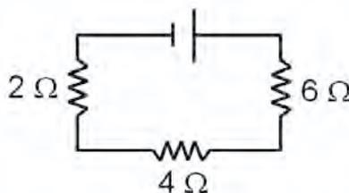
$$R_t = R_1 + R_2 + R_3 + R \dots$$
