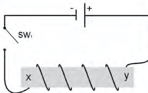
30. Based on the diagram above, which of the following statements describes the quantities induced into the iron core when  $SW_1$  is closed?
