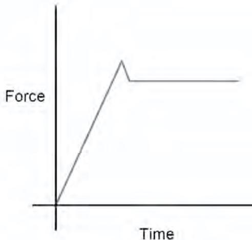
As we see in the graph above, more force is required to start an object in motion than is required to keep the object in motion.
