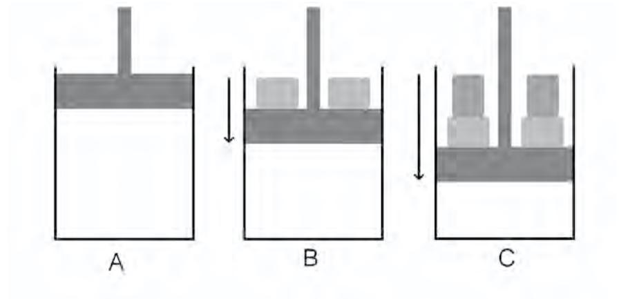
The diagrams show a gas enclosed in a cylinder that has a movable piston. Diagram A shows the gas under normal conditions. If we add weight to the outside of the piston in Diagram B, the pressure exerted on the enclosed gas is increased and its volume is reduced. In Diagram C, we add even more weight to the piston and the pressure on the gas increases again. The pressure and volume of the enclosed gas are indirectly related.
