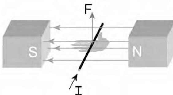
The diagram above shows a current carrying a magnetic field. According to the right-hand rule, the wire will experience a force in the upward direction. When the force exerted on a wire in a magnetic field is known, the magnetic field ( $B$ ) can be determined.
