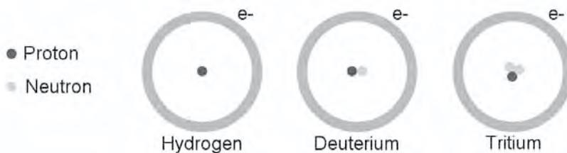
Notice that the hydrogen, deuterium, and tritium (above) each have one proton and one electron. The difference between them is the number of neutrons in the nucleus. The sum of the protons in a nucleus plus the number of neutrons is called the mass number, or ( $A$ ) number. Elements with the same atomic number but a different mass number are called isotopes.
