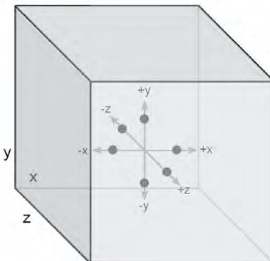
The particles of a gas in a closed container move in a random manner. However, there is a certainty that the enclosed gas molecules are moving toward or away from one of the walls of the container. Eventually, the gas particles strike one of the sides of the container. The impact each particle exerts on the container wall is its *momentum*, which is a product of the particle's mass and its velocity.
