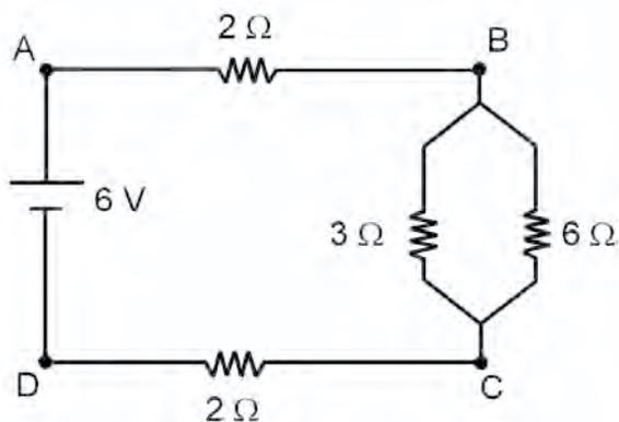
56. What is the resistance in the parallel circuit above between points *B* and *C*?
