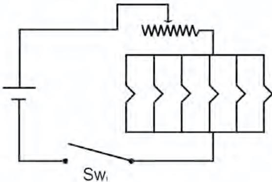
56. The diagram above shows a battery and a variable resistor set at its midpoint resistance in series with a parallel light circuit. Switch 1 ( $SW_1$ ) is closed and the light bulbs illuminate. When the variable resistor is moved slightly to the left ( $L$ ) the bulbs dim a little. When the variable resistor is moved slightly to the right ( $R$ ) the bulbs brighten slightly.
