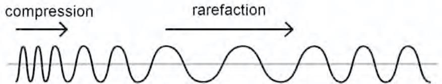
A Slinky held at both ends can be used to illustrate longitudinal mechanical waves. Compressing the spring (*c*) and then releasing it allows the compression to travel down the spring. Stretching the spring and releasing it would cause a stretched area or rarefaction (*R*) to travel through the spring in a similar way.
