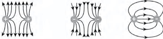
The field lines of the like charges do *not* cross one another, which produces repulsive forces. The field lines of the unlike charges work concurrently, producing an attractive force.
