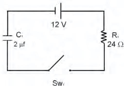
$C_1$  is an uncharged capacitor (shown in the circuit above). At  $t = 0$  the switch ( $SW_1$ ) is closed, and  $C_1$  begins to charge.
