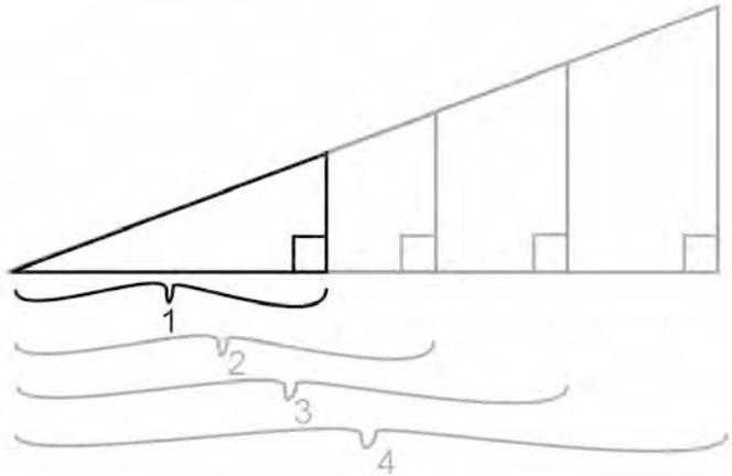
Triangles 1, 2, 3, and 4 above all have an internal angle of  $30^\circ$ . Thus the sine, cosine, and tangent values are the same in all four triangles.
