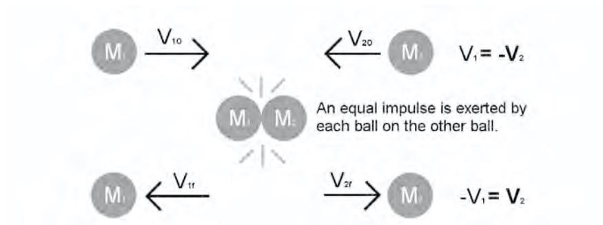
After the collision  $v_{1o}$  equals  $v_{2f}$  and  $v_{2o}$  equals  $v_{1f}$ . The momentum of each pool ball before the collision is the same as their momentum after the collision. Momentum is conserved, leading to the statement of the Law of Conservation of Momentum.
