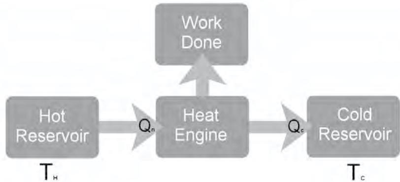
The flow chart above shows a generalized diagram of a heat engine. Heat from the hot reservoir ( $Q_H$ ) flows from a high temperature area to a low temperature area. Between the two areas some of the heat energy is used to do work. The remaining heat ( $Q_C$ ) becomes the exhaust.
