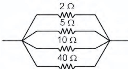
$$\frac{1}{R_t} = \frac{1}{2\Omega} + \frac{1}{5\Omega} + \frac{1}{10\Omega} + \frac{1}{40\Omega}$$
