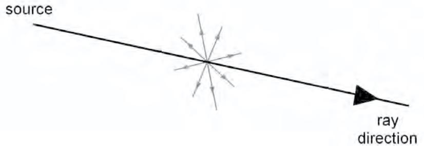
The polarized eyeglasses many people wear restrict the intensity of the light that reaches their eyes by using a device (polarizer) that only allows light vibrating on one plane to pass through to the eye.
