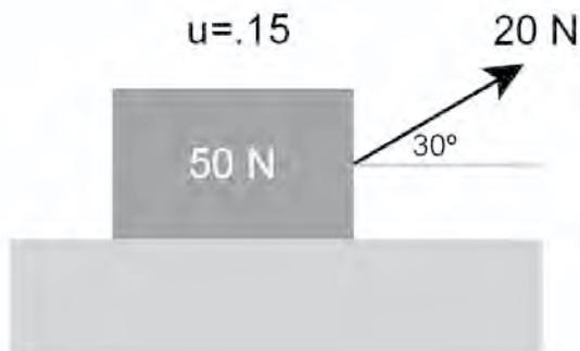
31. A block resting on the surface shown above has a force of 20N applied. Which statement best describes the force between the block and the surface upon which it rests?
