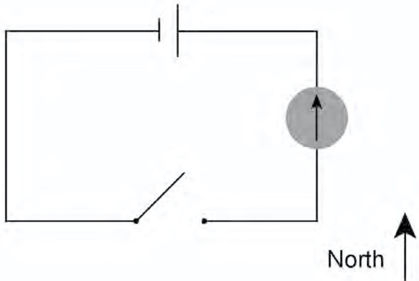
Notice that with the switch open the compass points correctly to the north. When the switch is closed the compass points in a different direction.
