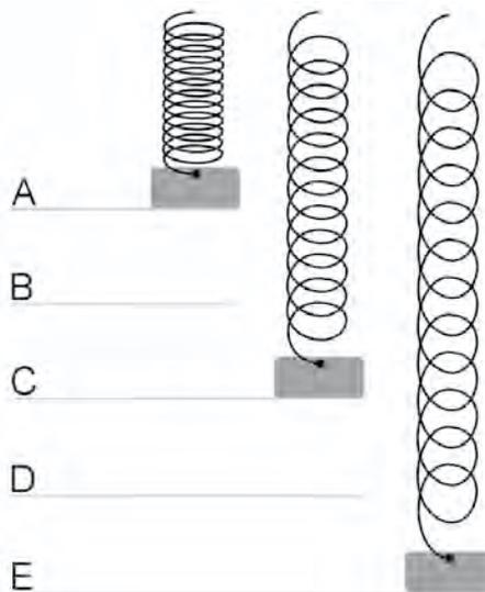
43. The hanging spring shown above has a mass attached to it. The spring is set in motion by displacing the mass downward and releasing it. At which point is the kinetic energy of the mass the greatest value? (Point A is the maximum compression of the spring, and Point E is the maximum expansion of the spring.)
