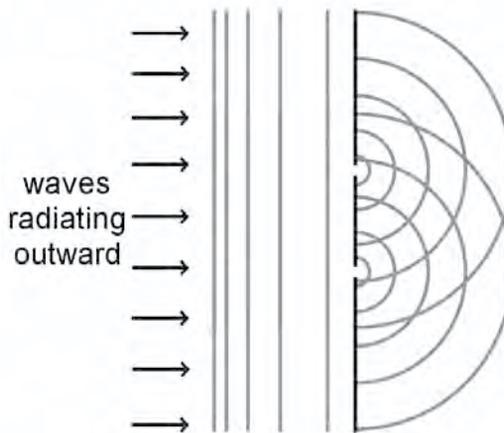
The area of waves beyond the barrier is filled with a confusion of waves crossing one another. A series of peaks and troughs exists as waves both constructively and destructively interfere with one another.
