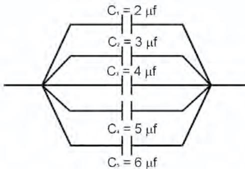
The six capacitors in the diagram have values of 2, 3, 4, 5, and 6 micro farads, respectively. The total capacitance is found by adding them together.
