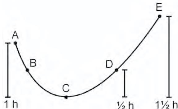
66. A 50 gram bead slides on a frictionless wire as shown above. At what point on the wire will the bead come to a complete stop?
