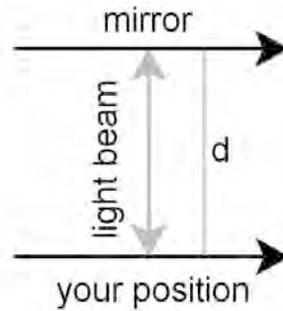
The distance  $d$  is the separation of the two sides of the car, yielding  $\Delta t = \frac{2d}{c}$  for the round trip.
