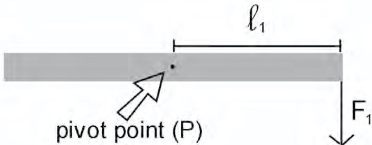
The uniform rod above weighs 2N and is 1m long. The force  $F_1$  is applied at the end of the rod, as shown. The lever arm  $\ell_1$  is the distance from the force  $F_1$  to the pivot point  $P$ . Should values of 10N be added for the force and a length of .5m for  $\ell$ , the calculation of the torques becomes:
