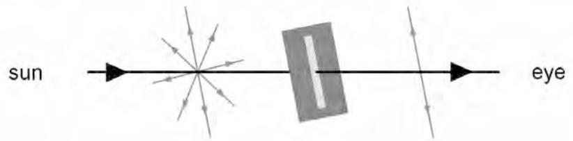
The result is similar to holding a meter stick over a rope that is vibrating up and down, but with the plane polarizer, every plane but one is polarized at the same time.
