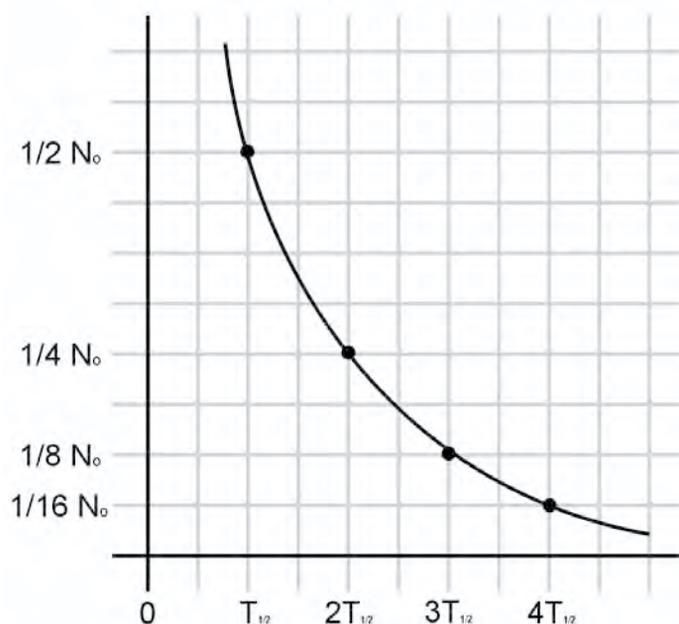
The graph above tells us that one half of a radioactive element has decayed away after one half-life. After two half-lives, 25% of the substance remains, after three it is 12.5%, and so on. After six half-lives, the radioactive material decays to negligible amounts. The remaining percentage of a radioactive substance after six half lives is calculated as follows:
