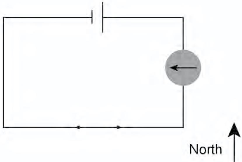
A force must affect the compass to cause it to point in a different direction. The current in the wire is the source of this force. The direction of the magnetic field around the current-carrying wire can be found by using a variation of the right-hand rule.
