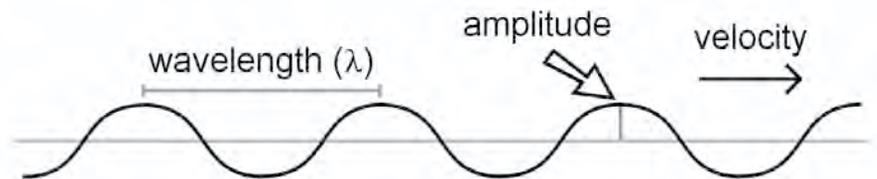
The drawing above shows a set of water waves moving past a fixed point. The wavelength ( $\lambda$ ), or distance between waves, is defined as the distance from any point on one wave to the same point on a following or a preceding wave. The rate at which the waves move past the point is their velocity ( $v$ ), and the number of waves occurring during a given time (number per sec) is the frequency ( $f$ ).
