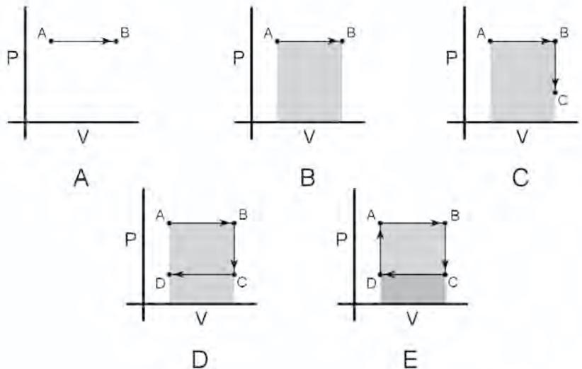
Diagram A shows an enclosed gas expanding at constant pressure. The piston moves outward and the system does positive work. The quantity of work done is equal to the pressure and the change in volume ( $P\Delta V$ ) and is the area under the  $P$ - $V$  curve. To do additional work, the piston must be able to repeat the process, but if the piston
