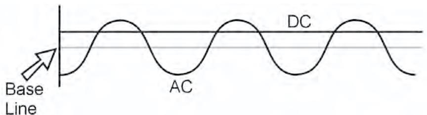
The AC peaks rise above the DC voltage because the effective voltage is equal to .707 the value of the maximum voltage. This is called the *RMS value*.
