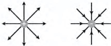
The positive test charge is repelled from the positive charged point, and it is attracted to the negative point (called point charges).
