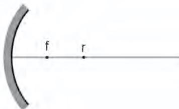
Concave spherical mirrors are important tools in science because of their ability to focus incident light. The point where incident rays are focused is called the focal point and is one half the radius of curvature.
