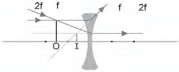
As with the mirror equation, the lens equations can be used to locate an image.
