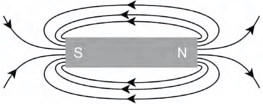
Magnetic field lines act much the same as electric field lines when magnetic poles are brought near one another. That is, *the magnetic lines of force do not cross*. You could say that the repulsive force the north pole of a magnet exerts on another similar magnetic pole is a manifestation of the lines of force not crossing one another.
