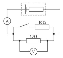
The cell has an e.m.f. of 1.5 V. The voltmeter reads 1.2 V when the switch is open.
