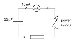
The capacitor is initially uncharged. The voltage across the power supply is then varied so that a current of  $10\,\mu\text{A}$  flows for 5.0 s.
